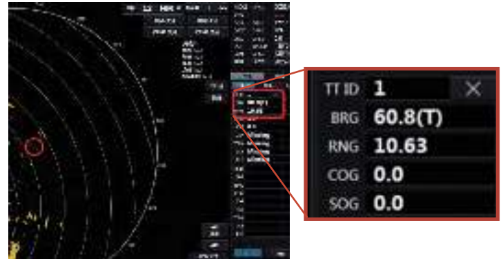
Detection range of a standard 10m 2 sphere at X-band (IMO standard 4.9NM))
